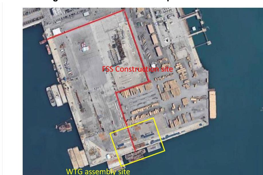
Once constructed a floating foundation is transferred onto a semi-submersible barge (see Figure 3-15 for example of semi-submersible barge construction site). This semi-submersible barge would be ballasted in order to progressively immerse the construction foundation up to the point that the foundation will float by itself. The foundation is then towed to the quayside (dockside) where the WTG assembly can start with components being erected on top of the foundation (see Figure 3-15).
